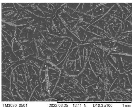
Fig. 2. Algae fibres on the paper surface SEM image, magnification 100x
